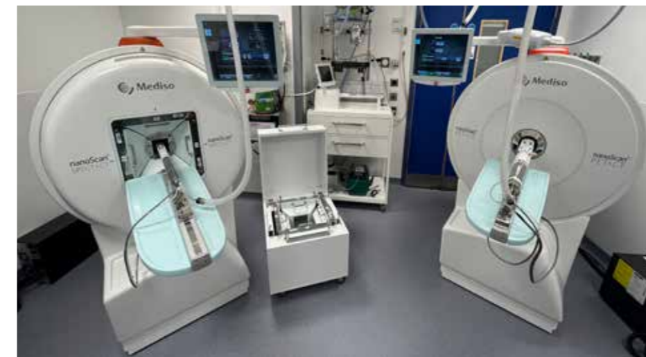
nanoScan® PET/CT and SPECT/CT reference installation of two systems in one small laboratory
